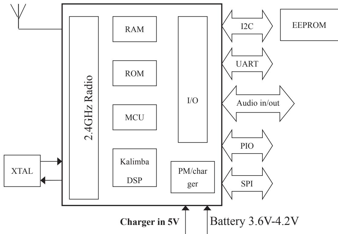
**Figure 1:** Block diagram of BTM-68D
