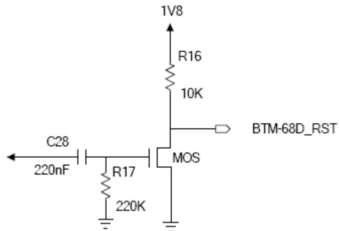
**Figure 2:** BTM-68D reset circuitry
