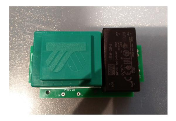
This model can deliver up to 4A on the 5V, so it's more than powerful enough to be used with 1541 Ultimate, 17xx Ram expansions, C128 with 17xx Ram expansion etc.
