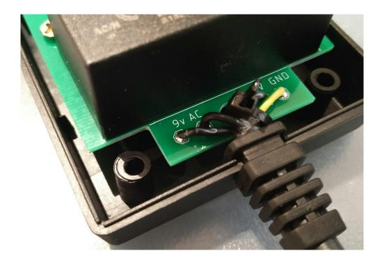
Screw in 4x3mm screws to fasten the PCB to the enclosue.
