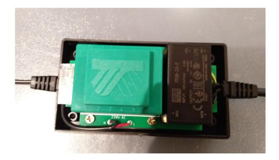
Put the plastic feet on each screw, close the enclosure, insert each screw into each hole in the bottom of the enclosure and screw in the screws till they are tight.
