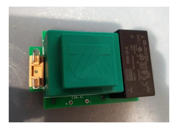
The fuse is a 500mA T 250V (slow burn) glass fuse. If you're having problems, or want to have a "C128" psu, you can upgrade it to a 500mA T 250V.
