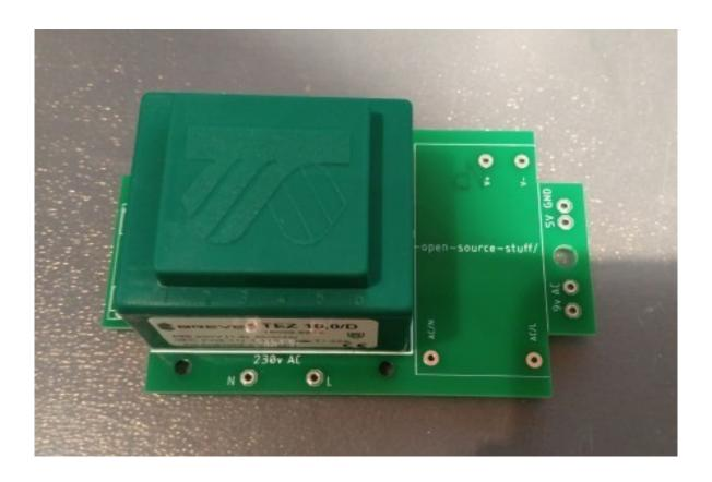
The trafo generates the 9v AC needed for the SID, if you measure the output you might get around 10v AC, thats fine. The voltage will drop once connected and powered on.
